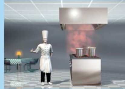
Picture 32. A wall model installed as an island model. In this case, overhang on the back is needed.
