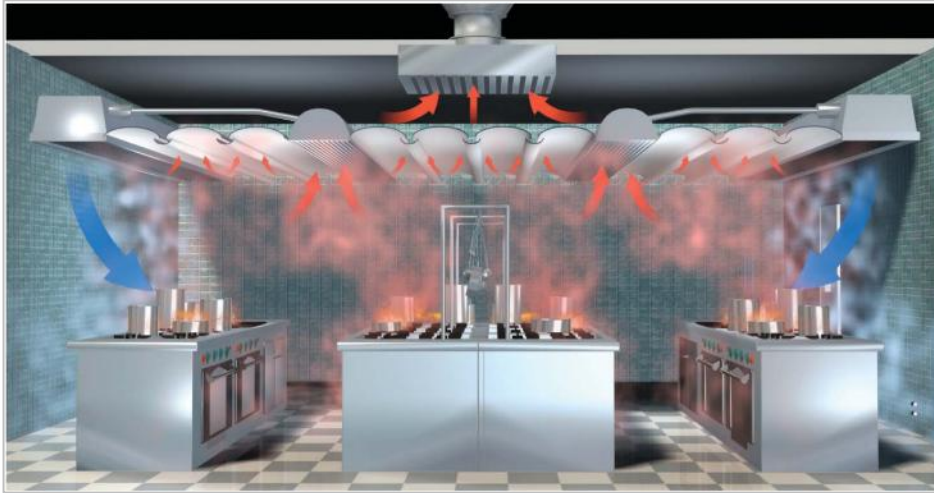
Picture 32. A wall model installed as an island model. In this case, overhang on the back is needed.
